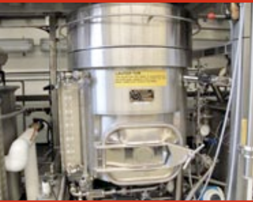
The liquid from the mash is separated from the solid husk material in the lauter tun pictured here. The liquid, called wort, flows to the kettle.
