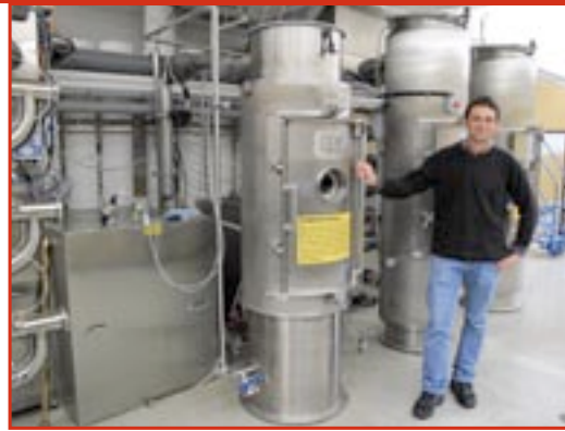
Mr Aleksandar Egi, malting and brewing specialist at the Canadian Malting Barley Technical Centre, introduces the steeping vessel which performs the first step of the malting process.
