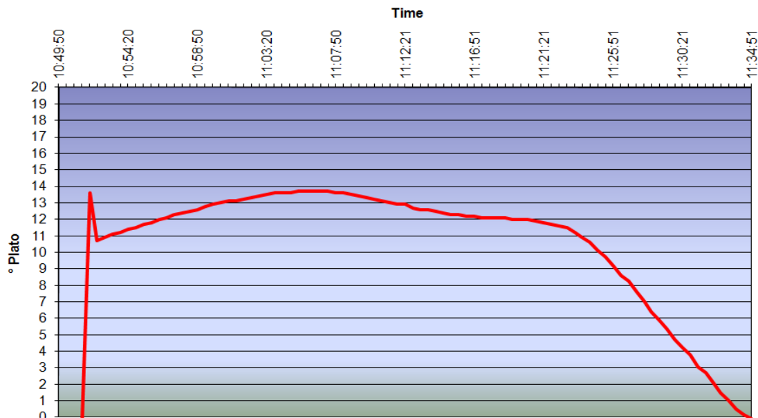
Figure 11: CDC Copeland runoff specific gravity profile for the 2012 QS test malts.
